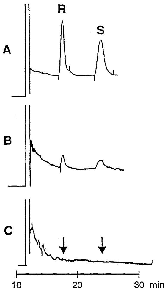
Fig. 6. Separation of diastereomeric almokalant glucuronides from direct injection of 50 \mu l of urine. (A) 30 \mu g/ml; (B) 0.5 \mu g/ml; (C) urine blank. Porous graphitic carbon (Hypercarb) was used as the separation column (100 \times 4.6 mm I.D.) and 30% acetonitrile containing 0.1 M acetic acid as the mobile phase [35].
